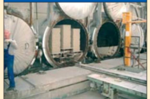
155 kg of steam at 12 bar to produce 1 m<sup>3</sup> of aerated concrete, which requires about 87 kWh of thermal energy. Generally, the steam is provided by steam generators with an output range of 5–10 MW. Ruths storage tanks are used for intermediate storage of waste heat.
