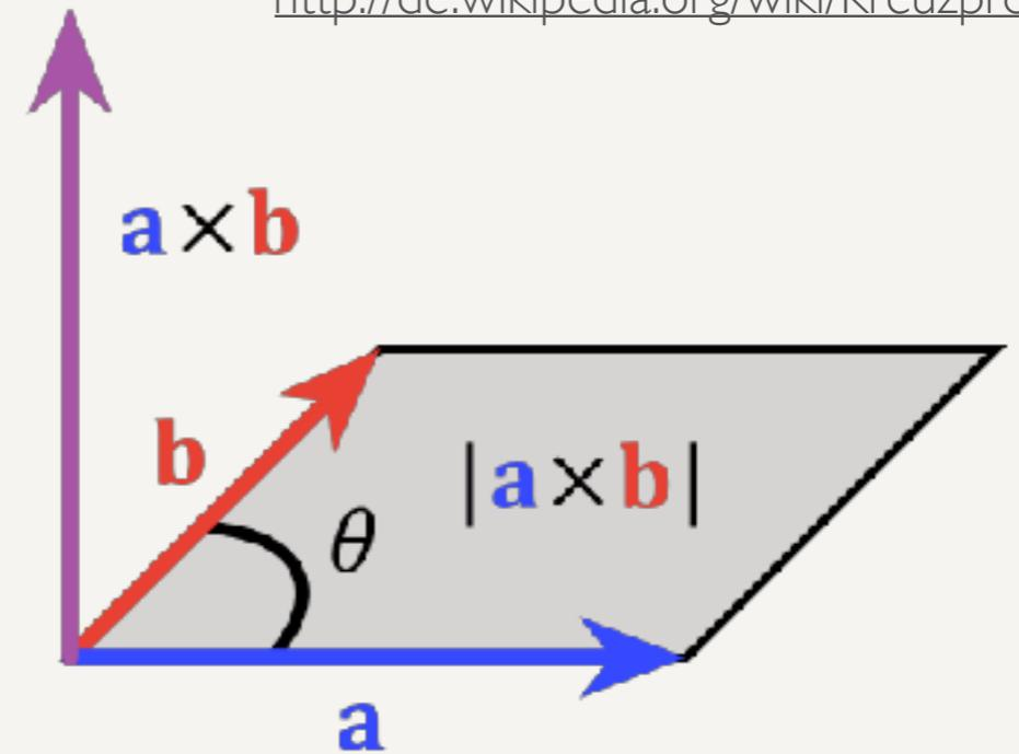
$$\begin{pmatrix} c_x \\ c_y \\ c_z \end{pmatrix} = \begin{pmatrix} a_x \\ a_y \\ a_z \end{pmatrix} \times \begin{pmatrix} b_x \\ b_y \\ b_z \end{pmatrix} = \begin{pmatrix} a_y b_z - a_z b_y \\ a_z b_x - a_x b_z \\ a_x b_y - a_y b_x \end{pmatrix}$$
